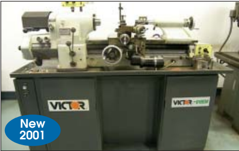
VICTOR #618-EM PRECISION TOOLROOM LATHE
