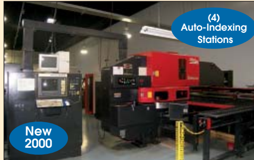
AMADA #PEGA-358-S CNC TURRET PUNCH WITH FANUC CONTROLS
