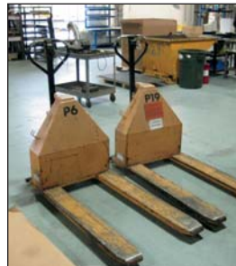
MULTITON #TMCX 5500 LB ELECTRIC PALLET TRUCKS
