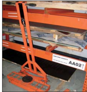
STEERMAN #S-25 MACHINE MOVING DOLLY SYSTEM
