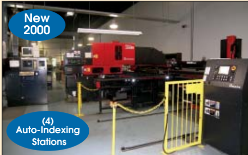
AMADA #PEGA-358-S CNC TURRET PUNCH WITH SHEET LOADING SYSTEM (May be sold separately)
