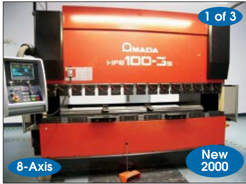
VIEW OF AMADA PRESS BRAKE 8-AXIS CNC CONTROLS
