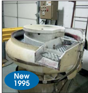
TIMESAVER #ZA-300 VIBRATORY FINISH MACHINE WITH UNLOADER
