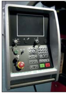
VIEW OF AMADA PRESS BRAKE 8-AXIS CNC CONTROLS
