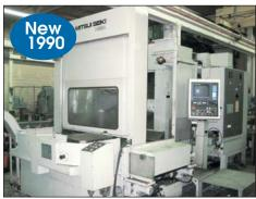
MITSUI-SEIKI MODEL HS-5A "5-AXIS" HORIZONTAL MACHINING CENTER, FANUC 15M, #CT-50 TAPER
