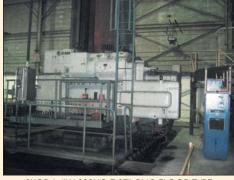
SKODA #W-200HC 7.87" CNC FLOOR TYPE HORIZONTAL BORING MILL
