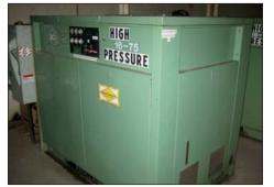
SULLAIR ROTARY SCREW AIR COMPRESSOR #16-75
