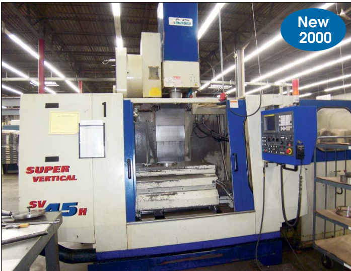
Johnford #SV-45H Vertical Machining Center
