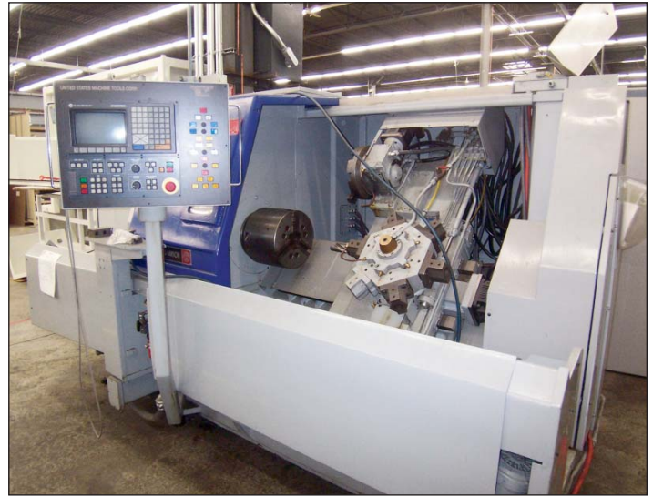
Jones & Lamson #TNC-A Slant Bed Turning Center
