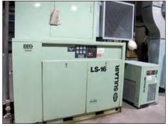
SULLAIR ROTARY SCREW AIR COMPRESSOR MODEL LS-16
