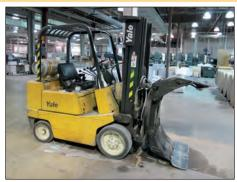
YALE 5000 LB LPG FORKLIFT, TRIPLE MAST W/ROLL CLAMP
