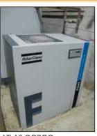
ATLAS COPCO COMPRESSED AIR DRYER MODEL FD-95
