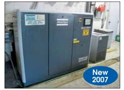
ATLAS COPCO ROTARY SCREW AIR COMPRESSOR MODEL GA22VSDFF7
