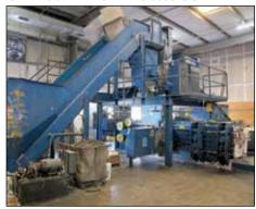
BALEMASTER HORIZONTAL BALER #AT-1-40 W/SHREDDER AND LOADER
