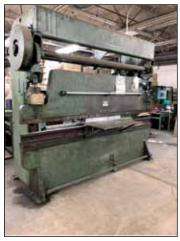
VERSON 10'- 65 TON PRESS MOD. 208-AUTOMEC CNC 9X9 CONTROLS
