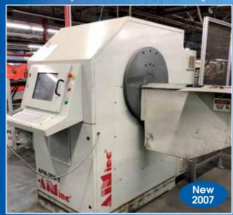
AIM Model AFM-3D8-T CNC Wire Former
