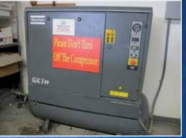
Atlas Copco Rotary Screw Air Compressor Model GX7-FF
