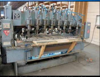
Lors 8-Station Welder Machine MW1 w/ Entron Controls
