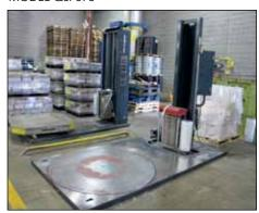
LANTECH & WULFTEC ROTARY STRETCH PALLET WRAPPERS
