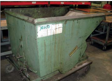
DUMPING SCRAP HOPPER
