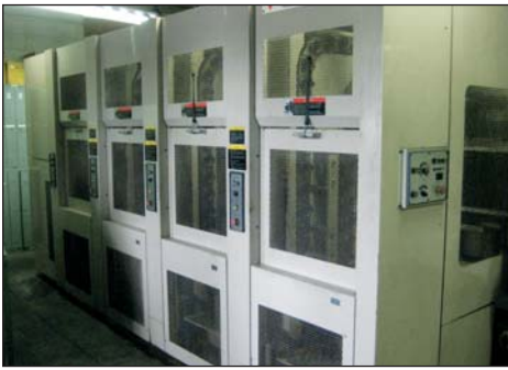
VIEW OF YASDA # YBM-700-6AP CNC HMC TOOLCHANGER (120) CAP.
