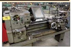
CINCINNATI 12 1/2 X 36 LATHE W/ 10" 4-JAW CHUCK
