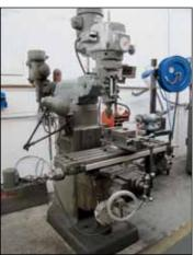
BRIDGEPORT 1.5 HP VERTICAL MILL, POWER FEED
