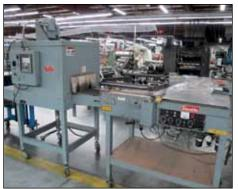
SHANKLIN L-SEAL PACKAGING MACHINE WITH HEAT SHRINK TUNNEL
