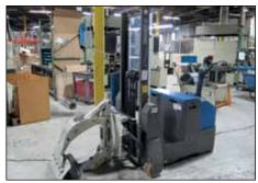
Armani Model DCP100/Walk Behind Pallet lift //Cascade Barrel Clamp, 2425 Lb,@21"
