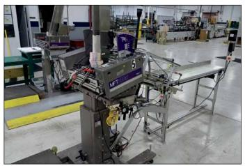
(8)MTF Friction Feeders/Delivery Conveyors, Models: MTF550 & MTF350;
