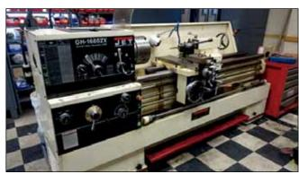
Jet 17/25" x 40"/60" Centers Gap Bed Lathe
