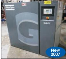
ATLAS COPCO 50 HP ROTARY SCREW COMPRESSOR MODEL GA37
