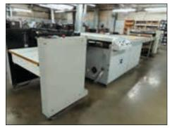
TEC LIGHTING UV CURING TUNNEL MODEL TC4548-1/16-A
