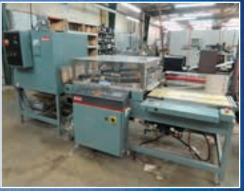
Shanklin L-Seal Packaging Machine Model A27A
