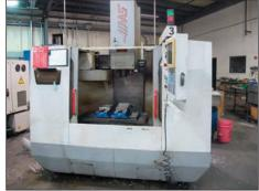
HAAS VF1 CNC VERTICAL MACHINING CENTER
