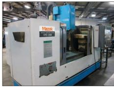
MAZAK VTC-20B CNC VERTICAL MACHINING CENTER
