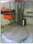
LANTECH Q-SERIES ROTARY STRETCH PALLET WRAPPER
