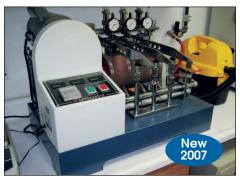
Hung TA Instruments Abrasive Tester Apparatus Model HTS-8621,
