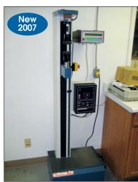
Hung TA Instruments Tensil Tester Model HT8336-S
