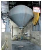
175 CuFt Patterson Kelly, Jacketed Conical Rotary Blender Vacuum Dryer
