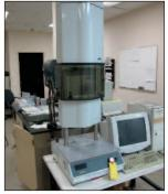
Kayness Capillary Rheometer Montano Rheometer Model D6052M-115
