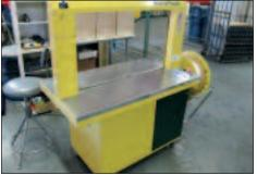
Strapack Automatic Strapping Machine Model RQ-8
