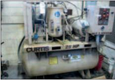
Curtis 25 HP Rotary Screw Compressor Model RS25A
