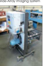
MBO Air Knife Fold Attachment Model Z2
