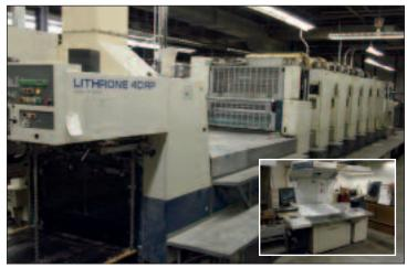
Komori L640RP-III Sheet Fed Printing Press / Komori L640RP-III Console
