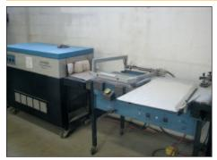
Weldotron Auto Shrinkwrap Machine Model 1602
