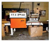
BELCO L-SEAL PACKAGING MACHINE W/HEAT SHRINK TUNNEL
