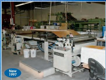
TUNKERS SEMI AUTOMATED MOUNTING MACHINE
