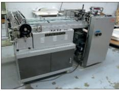
**ROLLEM SCORING & PERFORATING** MACHINE MODEL T.R.
