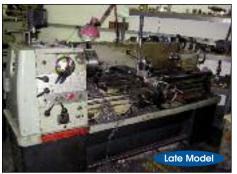
Clausing 15"x 60" "Gap Type" Engine Lathe
