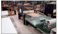
EASTEY 32" SHRINK WRAP PACKAGING MACHINE W/HEAT TUNNEL
