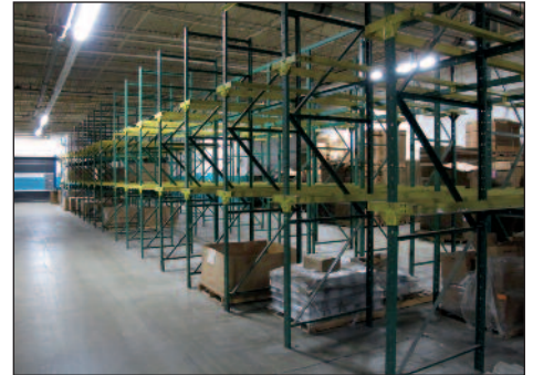
View of Push Back Pallet Racking
