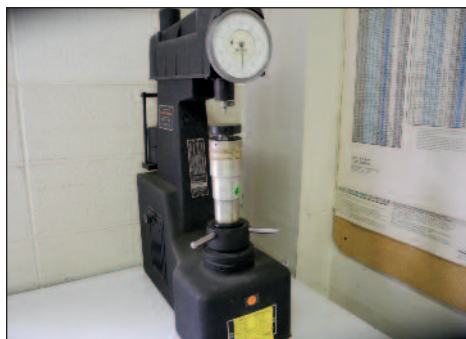
Rockwell Hardness Tester Model 3TBB
