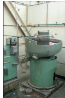
Roto-Finish #FT-8 Vibratory Finishing Mill
