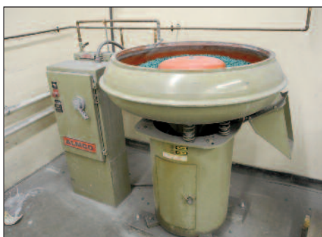
Almco Vibratory Finishing Mill Model OR-3
