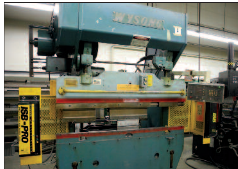
Wysong Mechanical Press Brake Model 55-4
