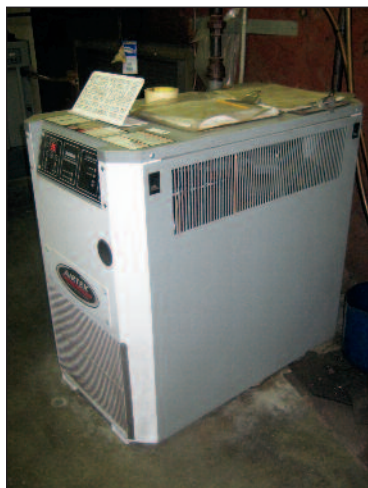
Airtek Refrigerated Air Dryer, Dual Mode, Model C130
