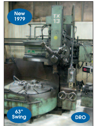
SHIBAURA # TX-13 "OPEN SIDE" VERTICAL TURRET LATHE
