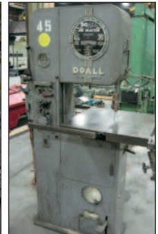
DO-ALL # ML 16" W/ Blade Welder-Grinder
