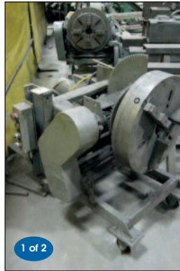
WORTHINGTON # 5-H, 500 lb Cap., Tilting Type W/ Chuck
