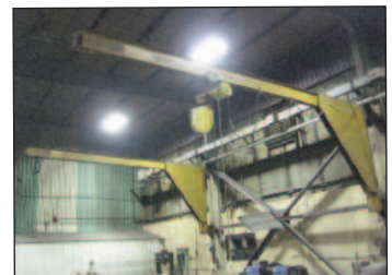
(28) MODULAR 12'-16' "BOLT ON TYPE" JIBS W/ Hoists
