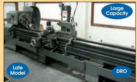
LEBLOND REGAL # SERVO-SHIFT ENGINE LATHE W/ 30"x 240" Cap
