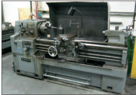
MORI-SEIKI # MS-1250 ENGINE LATHE W/ 17"x 50" Cap
