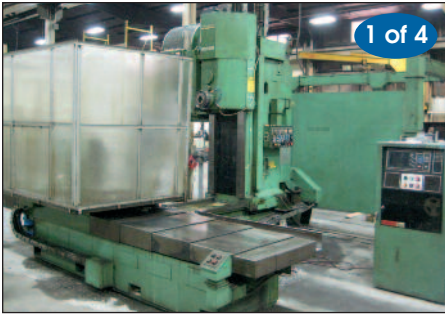
CINCINNATI # 10HC-1500 CNC "4-Axis" HORIZONTAL MACHINING CENTER
