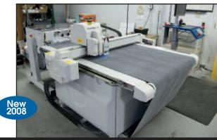
Kongsberg/iCut Finisher Model iXE10, Active Cutting Area 31" x 43", i-Cut Camera; i-Cut Vision Pro; i-Script, i-Cut Workstation w/ PC and Operator Panel; Kongsberg Table w/ Air Compressor, Vacuum Pump; Multi Function Unit w/ Measuring Probe, Ballpoint Pen Tool, Laser Pointer; VariCut Tool w/ T16 & T17 Knife Blades; XE Crease Tool; Conveyor System; Sheet Feeder w/ Pick & Place System, Loading Table & Material Guide;
