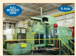
SNK # FSP-100-V "5-Axis" CNC Horizontal Machining Center
