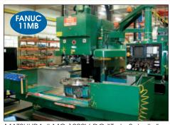
MATSUURA # MC-1000V-DC "Twin Spindle" "4-Axis" CNC VMC
