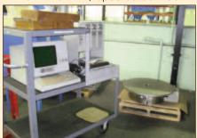
PNEUMO AIR BEARING ROTARY GAGE W/ Controls
