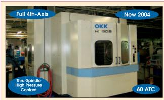
O.K.K. # HM-80-S CNC Horizontal Machining Center
