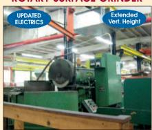
ARTER # B-30, 30" Horizontal Spindle Rotary Surface Grinder W/ 31" Dia. Magnetic chuck, Tilting Table, Swing 41", Max. Work Height 18", Wheel Size 20", Coolant System S/N 1106
