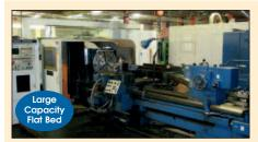
AMERICAN "Flat Bed" CNC Lathe W/34" x 108" Cap., 21" 3-jaw Chuck, Tailstock, 5-station & 4-station Turrets & General Automation CNC Control, S/N 80033/73 ☞
