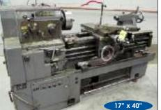
Webb #WL-435 "Gap Type" Engine Lathe
