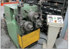
Eagle Tube Bending Machine Model
