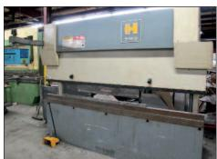
Haco CNC 10' x 120-Ton Euromaster Hydraulic Brake Model SRM-120-10
