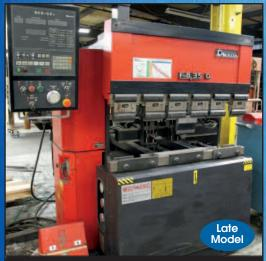
Amada CNC 4' x 35-Ton, Hydraulic Press Brake Model FBD3512E
