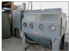
Trinco Mod.# 6044 Dual Station Dry-Blast Cabinet W/Dust Collector
