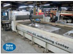
Omax CNC Waterjet System Model 80X
