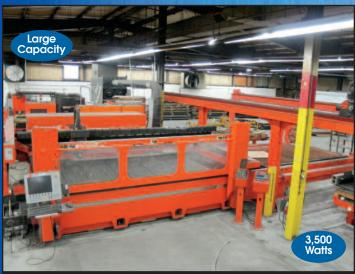
Bystronic Laser Cutter Model BTL3500
