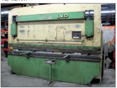
LVD 12' x 200-Ton Hydraulic Power Press Brake Model PPBL200-40
