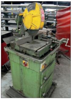
Doringer Model D350 Heavy Duty Cold Saw
