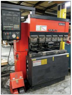
Amada CNC 4' x 35-Ton, Hydraulic Press Brake Model FBD3512E
