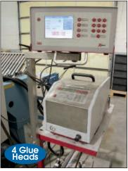
HHS Promelt Hot Melt Glue System Model HMP-04-1X4PDE
