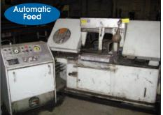
Marvel Hydraulic Horizontal Band Saw, Model 15A4/M1
