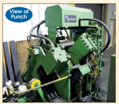
FICEP CNC Hydraulic Angle Punch & Shear Line
