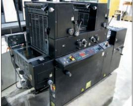
AB Dick 2/C Offset Press #9985, S/N L8492, Crestline Dampening, Airtech Ultra Air Powder System
