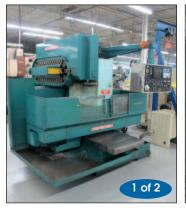
Matsuura #MC-760V CNC Vertical Machining Center
