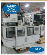
Kitamura #Mycenter-1 CNC Vertical Machining Center
