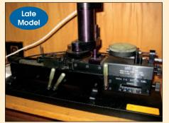
Vari-Roll #F-2 "Computerized" Gear Tester
