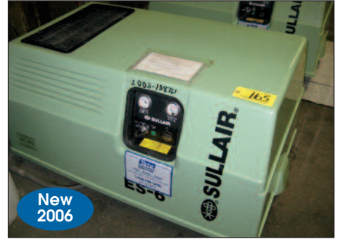
(2) SULLAIR # ES-6 ROTARY AIR COMPRESSORS
