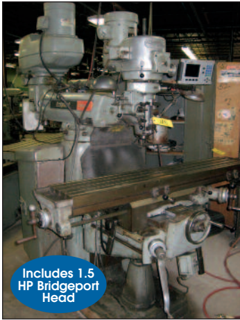
Bridgeport Series II "Special" 4HP Vertical Milling Machine
