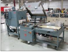
Shanklin #27A L-Seal Packaging Machine w/Heat Tunnel
