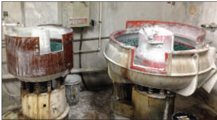
PARTIAL VIEW OF DEBURRING MACHINES
