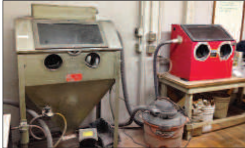
VIEW OF BLAST CABINETS
