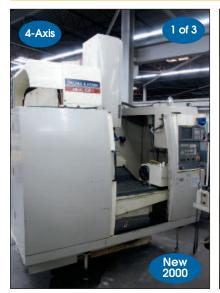
OKUMA & HOWA CNC VERTICAL MACHINING CENTER #MILLAC 438V, FANUC 18M CONTROL
