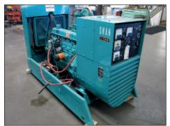
ONAN ELECTRIC GENERATOR SET # 30EX-30.0EK-15R/1786H, 3 PHASE, 35 KW, 1 PHASE, 20 KW, 725 HOURS
