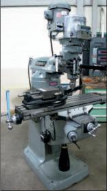
BRIDGEPORT 2 HP SERIES I VERTICAL MILL, S/N 243643, POWER FEED, ACCURITE DRO
