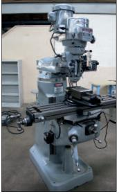
BRIDGEPORT 2 HP SERIES I VERTICAL MILL, S/N 141958, POWER FEED, SWI DRO
