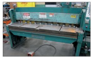
WYSONG SHEAR MODEL 1272, 12 GAUGE CAPACITY, 6'
