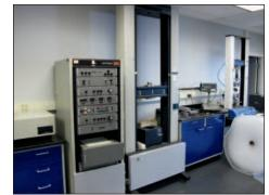
INSTRON LOAD CELL TENSILE TESTER MODEL 1125
