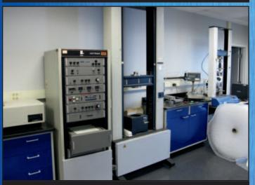
Instron Load Cell Tensile Tester Model 1125
