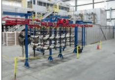
OVEN/DRYING CONVEYOR SYSTEM, 3-LANE OVEN, 230-280 DEG F TEMP
