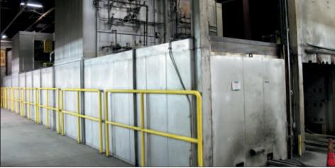
CUSTOM DESIGNED & FABRICATED 9-BURNER REFRACTORY MELTING FURNACE, 2,800°F TEMP
