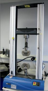
INSTRON LOAD CELL TENSILE TESTER MODEL 3369
