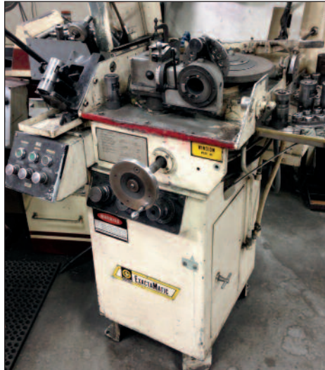
G&L "EXACTAMATIC-WINSLOW" # HC DRILL GRINDER
