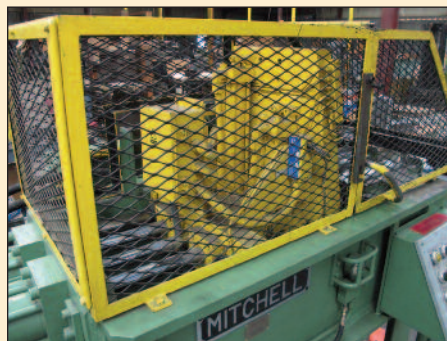
TUBE FORMING SYSTEM INCLUDING: (1) MITCHELL HYDRAULIC PUSH POINTER S/N PP-589 (NEW 1998), 33,000 LB. 3-DIE TUBE PUSH POINT & (2) MITCHELL HYDRAULIC PUSH POINT DRAWING MACHINES S/N PP-592 & PP-588 (NEW 2001), 60,000 LB. 3-TUBE EXTRUSION MACHINE
