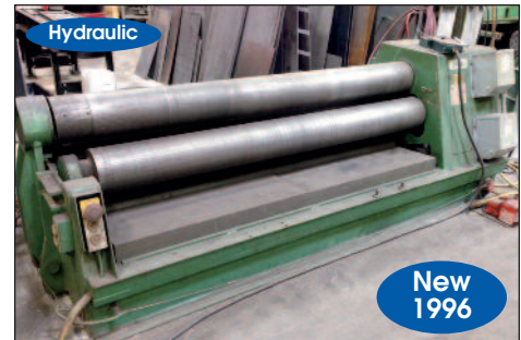
ROUND-AB # PS-205 HYD. PLATE BENDING ROLL W/ 6' X 3/8" CAP
