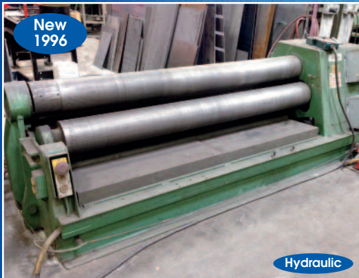
ROUND-O-AB # PS-205 HYD. PLATE BENDING ROLL W/ 6' X 3/8" CAP
