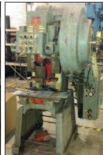
V.O. # 15-ST "HIGH SPEED" OBI PUNCH PRESS
