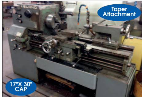
LEBLOND "REGAL SERVO-SHIFT" ENGINE LATHE
