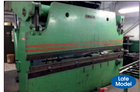
ACCURPRESS # 720012 HYD. PRESS BRAKE W/ 12' X 200 TON CAP
