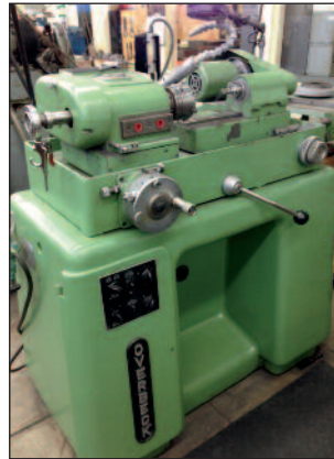
OVERBECK # ZETTO-30 "PRECISION" INTERNAL (I.D.) GRINDER
