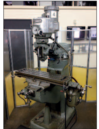
BRIDGEPORT 1.5 HP "VARIABLE-SPEED" MILLING MACHINE
