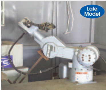
OTC-DAIHEN # FUSION ARC-100 ROBOTIC WELDING SYSTEM
