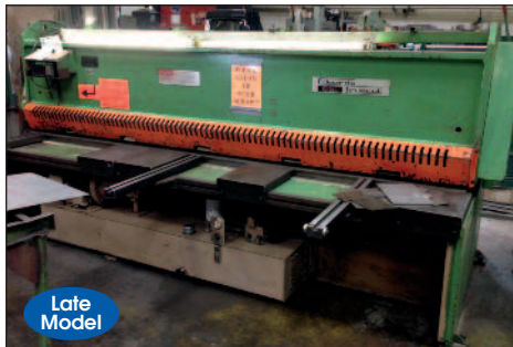
EDWARDS # 6.5-3000 "TRUECUT" HYD. POWER SHEAR W/ 10' X 1/4" CAP., F.O.P.B.G
