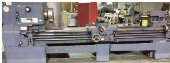
LEBLOND 26" X 96" "REGAL SERVO SHIFT" ENGINE LATHE
