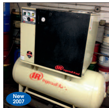
INGERSOLL-RAND 15 HP AIR COMPRESSOR MODEL # UP6-15C-125
