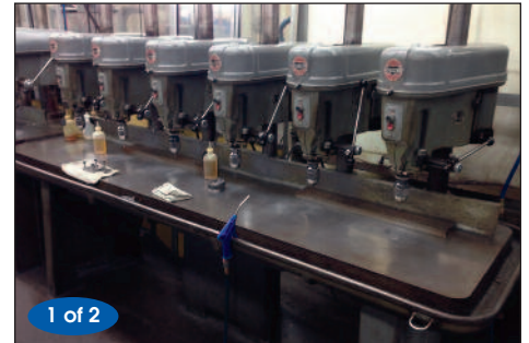
DELTA-ROCKWELL "6-SPINDLE" DRILL PRESS W/ H.D. 24" X 96" BASE & ALBRECHT KEYLESS CHUCKS
