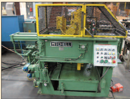
TUBE FORMING SYSTEM INCLUDING: (1) MITCHELL HYDRAULIC PUSH POINTER S/N PP-589 (NEW 1998), 33,000 LB. 3-DIE TUBE PUSH POINT & (2) MITCHELL HYDRAULIC PUSH POINT DRAWING MACHINES S/N PP-592 & PP-588 (NEW 2001), 60,000 LB. 3-TUBE EXTRUSION MACHINE
