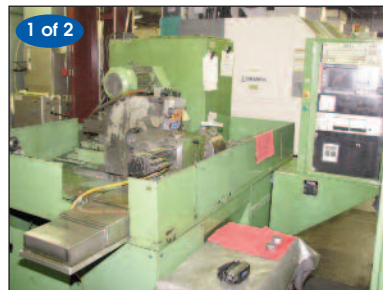
TSCHUDIN # HTG-52 "3-AXIS" CNC CYLINDRICAL GRINDER
