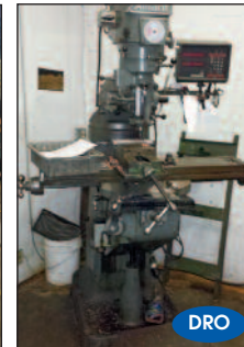
ALLIANT # RT-2 VERTICAL 2 HP MILLING MACHINE
