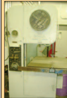
DO-ALL # ML 16" VERTICAL BANDSAW
