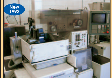
MITSUBISHI # DWC-90SB "4-AXIS" CNC WIRE EDM MACHINE
