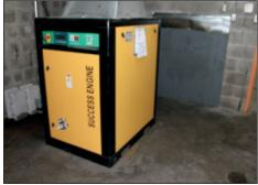
Success Engine 30 HP Air Compressor Rotary Screw
