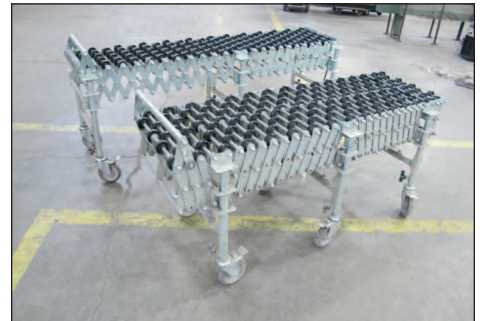
VIEW OF ACCORDING TYPE CONVEYORS
