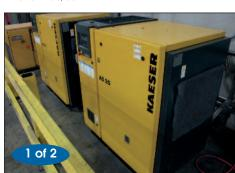
KAESER ROTARY SCREW AIR COMPRESSOR MODEL AS25
