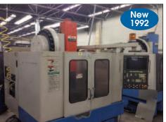
Mazak # MTV-414 CNC Vertical Machining Center
