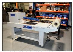
CLAMCO L-SEAL PACKAGING MACHINE MODEL 120-COMBO
